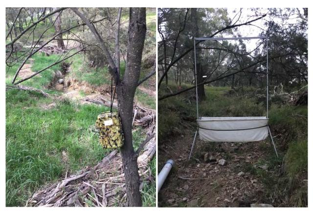
Figure 4-1 Harp and anabat set up for bat surveys in October 2019.
